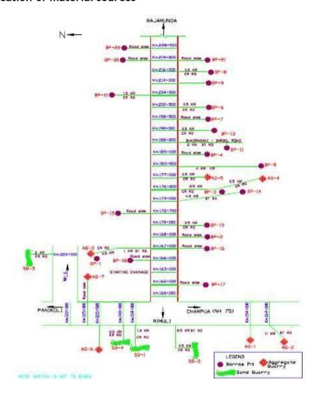
Figure 4: Key plan showing location of potential borrow pits tested
